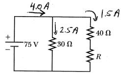
The current flowing through the battery is 4.0 A. Fill in the missing values in the table below.
