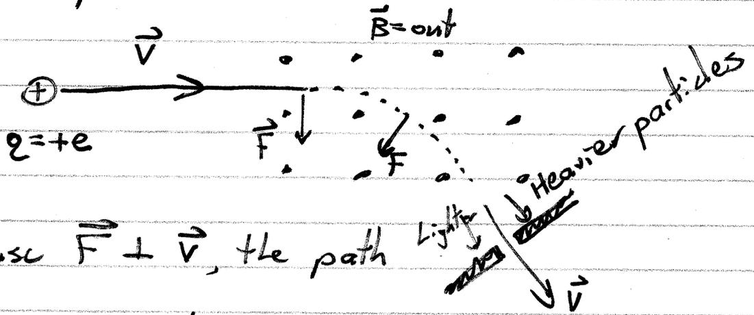
Because  $\vec{F} \perp \vec{v}$ , the path has a circular shape.
