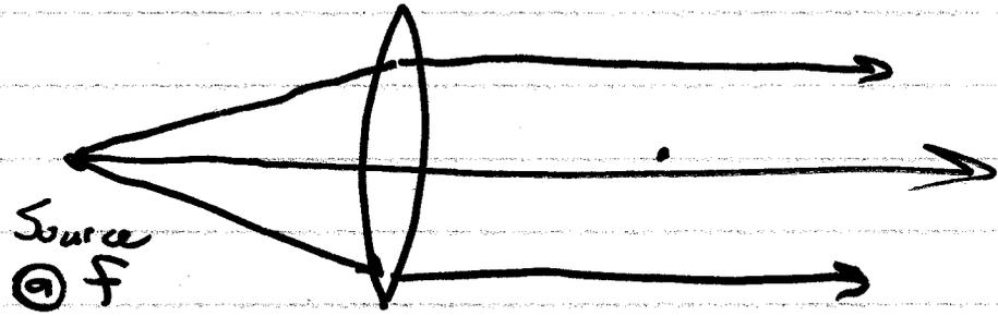
Object @ focal point makes parallel rays. Spotlight configuration.
