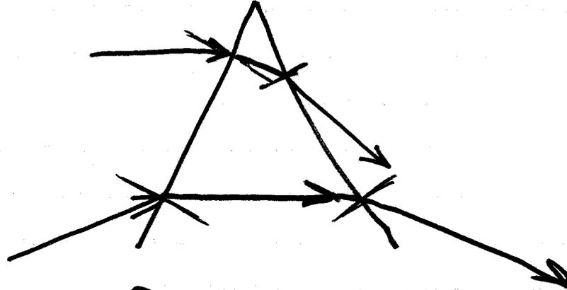
At both surfaces, the light bends away from the apex of the prism.
