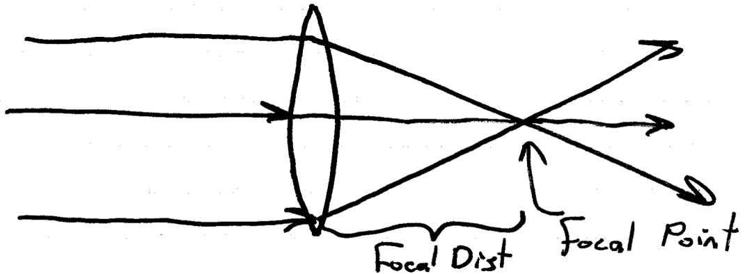
For a converging lens, Any "Parallel Ray" bends to the focal point.
