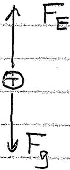
Need  $F_E = F_g = mg = (1.68 \times 10^{-6} \text{ kg})(9.8 \text{ N/kg})$
