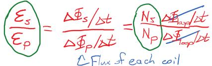
So the voltage ratio is the same as the turns ratio.
