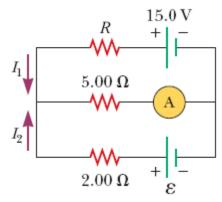
In the figure above,  $R=6.75~\Omega$  and the ammeter reads 1.85 A.
