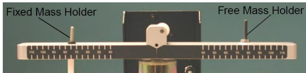
Figure 1: Rotating arm of the Centripetal Force Apparatus. The Fixed Mass Holder is held in place when masses are secured to the top. The Free Mass Holder can slide freely even when masses are secured in place. (Image from PASCO ME-8088 Instructions.)
