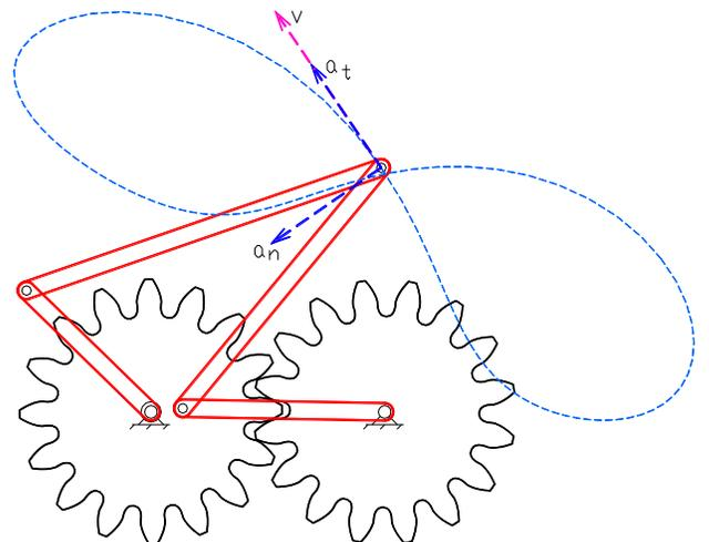
Figure A4: A geared-five bar linkage.
