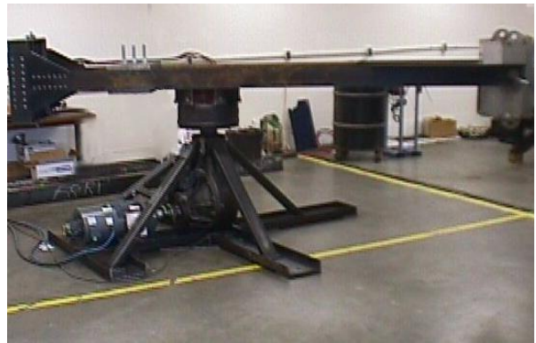
Fig. A2 Vertical axis 7ft radius centrifuge (client Auburn University Solidification Design Center)
