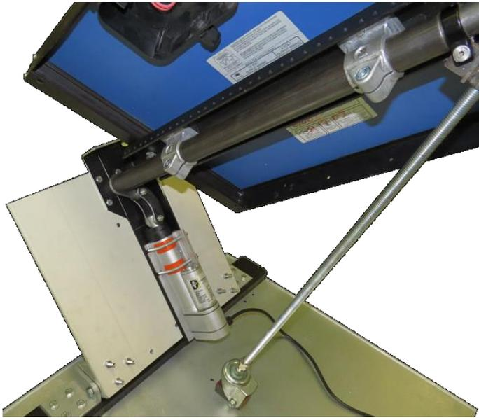
Figure 1: Single-axis solar tracking PV panel prototype.
