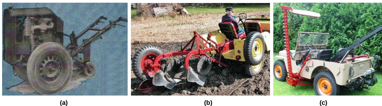
Fig. 3 – Walk-behind tractor fabricated using automobile components (a), and Jeep Willis automobiles equipped hydraulic three-point-hitches utilized as agricultural tractors (b) and (c).
