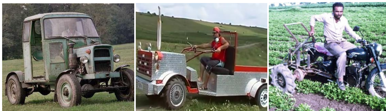
Fig. 4 – Contemporary automobiles and motorcycle converted in agricultural tractors and transport vehicles.
