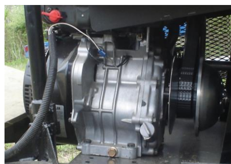
Fig. 6 – Details of a BUV equipped with continuously variable transmission (CVT). The manufacturing cost of such a vehicle is approximately 3000 US dollars.
