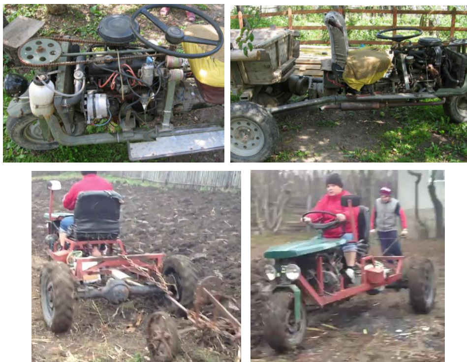
Fig. 5 – Homemade three-wheel tractors fabricated using salvaged DACIA and ARO components
