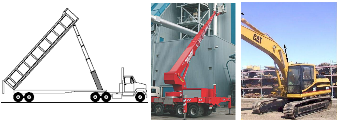
Figure 4: Examples of revertible elevating structures using: (left) one telescopic cylinder, (middle) single cylinder and (right) two parallel cylinders.
